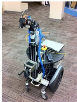
The robot platform used in this work is shown above. The 3D laser sensor can be seen at the top of the robot.
