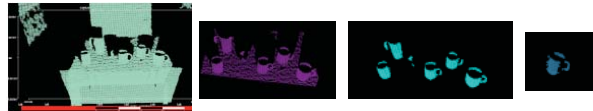
A visualization of the process to segment and extract objects from a point cloud.
