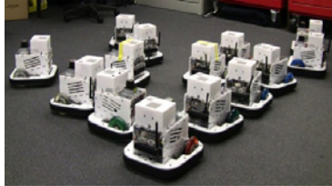
Figure 1b. Fleet of scarabs used to demonstrate multi-robot SLAM using wall features and door features in a distributed data fusion framework.
